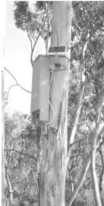
Figure 3. Bat box fitted with a wireless sensor unit.
