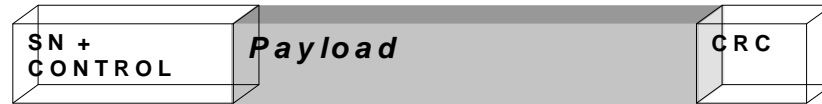
Figure 30. Representative frame structure for AAL small block ARQ system with variable payload.
